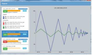
Figure 5. Degauss application for cryomodule magnets, currents versus time of SC solenoids and dipole correctors simulated with Virtual Accelerator.
