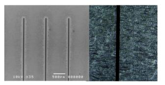
Figure 3: The SEM image of a standard multi-slit (left) with the Laser Scanned Microscope image (right). The LSM measurement yields  $47.4 \ \mu m$  as the width of the slits
