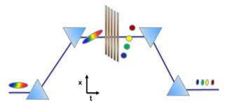
Figure 1: Schematic of the ASTA bunch compressor with the Z-Slicer.
