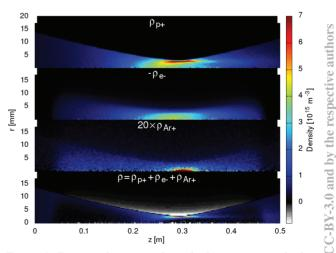
Figure 1: Proton, electron and residual gas ion particle densities in the simulation of the 50cm drift test system. The repeller electrodes at -1.5 kV are visible at the front and the back of the system.
