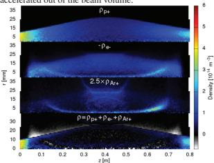
Figure 4: Particle densities for a system containing one solenoid 25 cm long at  $B_{max} = 378$  mT.
