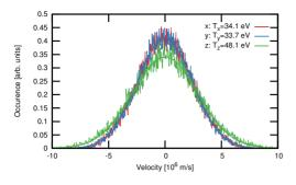
Figure 3: Electron spectrum at the center of the system in the steady-state.
