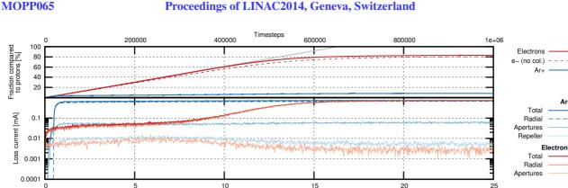
Figure 2: Particle population and losses during the built-up of space-charge compensation for the 50 cm drift system. The compensation degree is plotted for two different simulation runs: with and without electron induced ionization (dashed).
