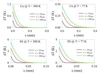
Fig. 7: Temperature profiles at the cavity surface at the end of specified pulse lengths.
