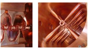
Fig. 1: IH - type (left) and CH - type (right) structure.
