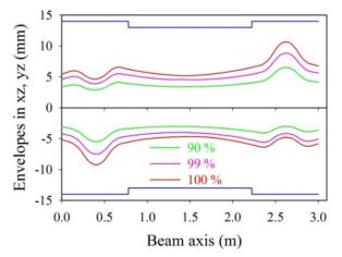
Fig. 2: Transverse beam envelopes along the 13.2 MV section for a 150 mA U28+ - beam.
