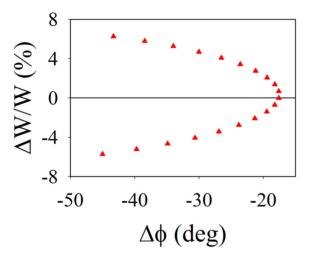
Fig. 3: RF phase of the bunch centre along the fixed beta profile with 20 gaps.
