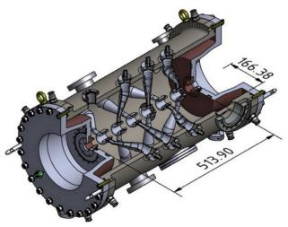
Fig. 6: 325 MHz high field prototype cavity with 7 gaps.
