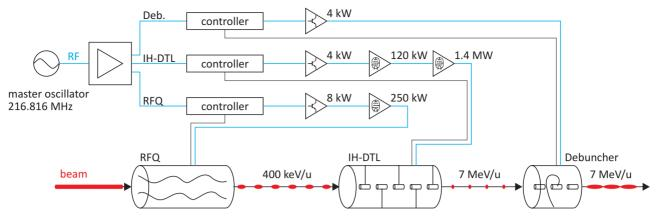
Figure 2: Schema of the LINAC RF System: One Master oscillator at 216.816 MHz, amplifier and divider distributes the RF to the three amplifiers, amplifier for the RFQ (8 kW transistor, 250 kW tube amplifier), amplifier for the IH-DTL (4 kW transistor, 120 kW tube amplifier, 1.4 MW tube amplifier), amplifier for the Debuncher (4 kW transistor). The control loop corrects amplitude and phase of the decoupled signal of the accelerator cavities.
