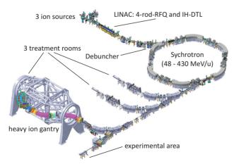
Figure 1: The accelerator of the Heidelberg Ion-Beam Therapy Center (HIT) with three ion sources, the LINAC (7 MeV/u) consisting of a 4-rod-RFQ and a IH-DTL, the synchrotron (48-430 MeV/u), the beam lines to the treatment rooms and the experimental area and the heavy ion gantry [1].
