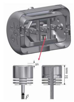
Figure 2: Dynamic 3-cell bellow tuner for the sc 325 MHz CH-cavity.
