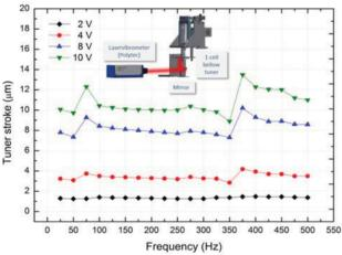
Figure 6: Measured tuner stroke as a function of the number of motor steps (top) and measurement results of the tuner stroke as a function of the applied piezo frequency for different operating voltages (bottom).
