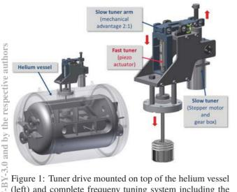
Figure 1: Tuner drive mounted on top of the helium vessel (left) and complete frequeny tuning system including the dynamic 3-cell bellow tuner (right).
