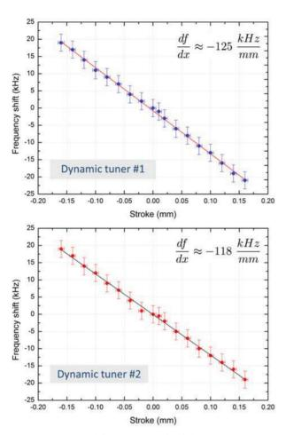
Figure 3: Measured frequency shift of the dynamic bellow tuners for the sc 325 MHz CH-cavity.
