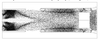
Figure 11: Slow ion distributions in the tube.
