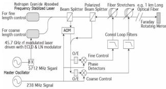
Figure 6: Optical-fiber length control system.
