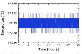
Figure 5: Temperature control performance of the 238 MHz sub-harmonic buncher. The temperature is regulated within +/- 2 mK (p-p).
