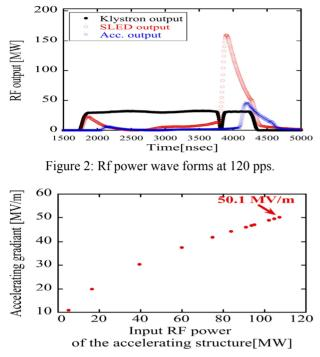
Figure 3: Acceleration gradients of the  $2\pi/3$  CG accelerating structure, as a function of its input rf powers. These gradients are calculated by using a shunt impedance of 64 M  $\Omega/m$ .
