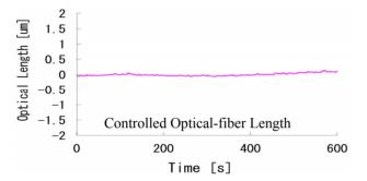
Figure 7: Control performance of the optical-fiber length control system. The fiber length is regulated within  $1\mu m$  in the case of only the fine control.
