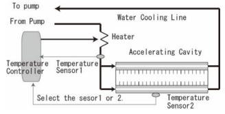
Figure 4: Highly precision cavity temperature controller.
