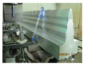
Figure 6: RFQ vane under machining process & cutter used
