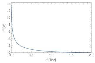
Figure 2: Integrated steady state wakefield power from f up to 2 THz generated by 300 pC 25  $\mu$ m bunches at 1 MHz in L3. Of the 13.8 W total lost by beam, about 50% is lost above 20 GHz, and 25% above 100 GHz.
