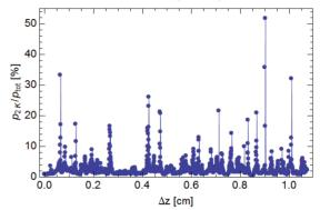
Figure 4: Percentage of power deposited at 2 K,  $p_{2K}/p_{\text{tot}}$ , vs. added cavity pipe length at f = 20 GHz.
