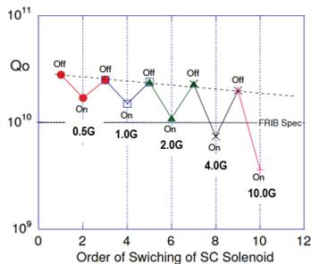
Figure 13: Q-drop depending on fringe field strength and Q-recovery by “quench annealing” process.
