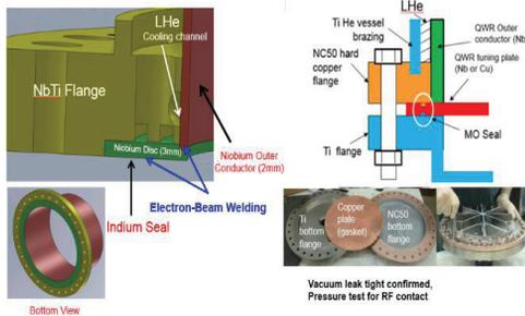
Figure 6: Redesigned bottom flange (left) with indium seal, and metal gasket bottom flange utilizing NC50 under development (right).
