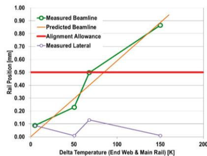
Figure 9: Alignment validation of bottom-up assembly in ETCM. Alignment error within 0.1mm is confirmed.
