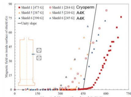
Figure 14: Saturation field of the cryogenic shield at 300 K and 10 K.
