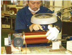
Figure 12: Dry winding (no epoxy used) at KEK
