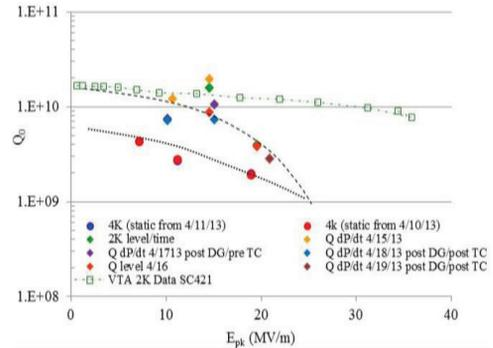
Figure 8: Cavity performance in the TDCM. Squares are baseline performance in the VTA test.
