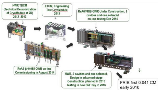
Figure 7: FRIB cryomodule prototyping approach.
