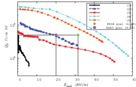
Figure 5: ReA3 QWR cavity performance in the early test.  $Q_0$  goes down at very low field, steep Q-slope is also seen.
