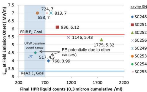
Figure 10: Good correlation between particle count and FE onset at FRIB QWR preparation.
