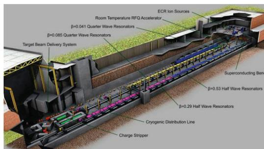
Figure 1: Linac configuration in FRIB tunnel.
