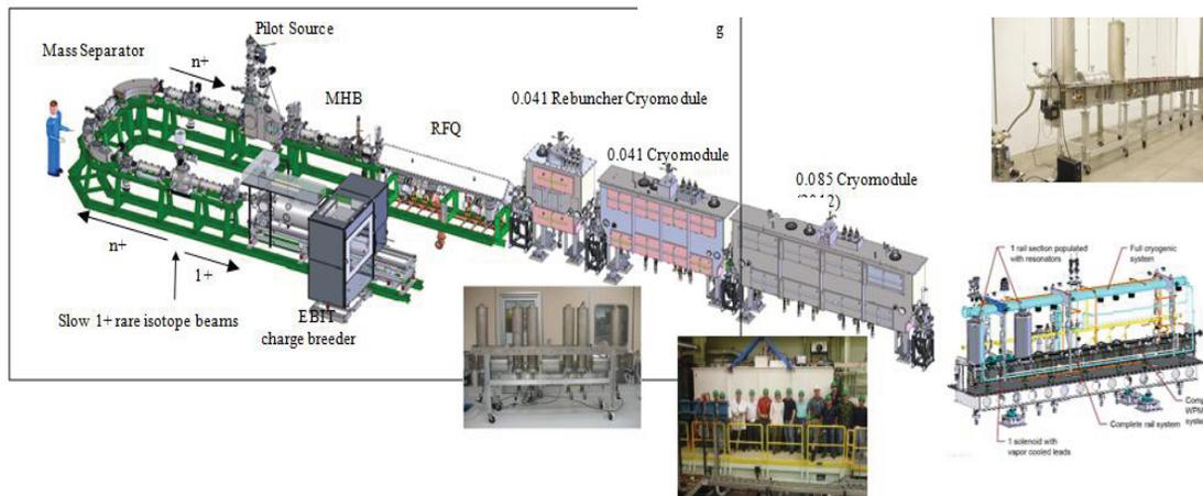
Figure 4: ReAproject in MSU. The box designates the existing system, CM#3 (pictured) is under commissioning and one more 0.085QWR cCM (right) which is exactly the same specification as the FRIB 0.085QWR CM, but including only two cavities and one solenoid. The coldmass assembly was completed in June 2014 and is now undergoing cryomodule assembly.
