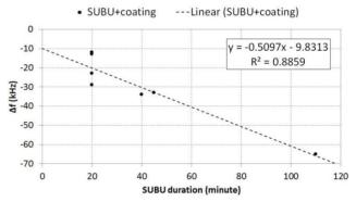
Figure 2: Correlation between resonance frequency shift and chemical polishing time.
