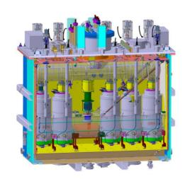
Figure 7: HIE-ISOLDE high-beta cryomodule.
