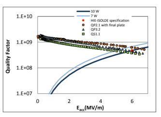
Figure 3: Performance of the first 3 series cavities. The red dot indicates the HIE-ISOLDE specification.
