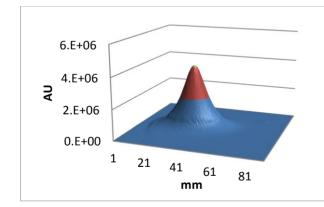
Figure 4: Beam footprint at the BLIP target for 130-µAbeam current.
