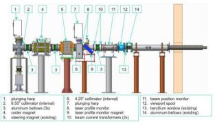
Figure 9: Proposed lay out of the last leg of the BLIP beam line.
