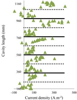
Figure 3: Current density distribution across an SPL 5 cell cavity from wall thickness measurements.
