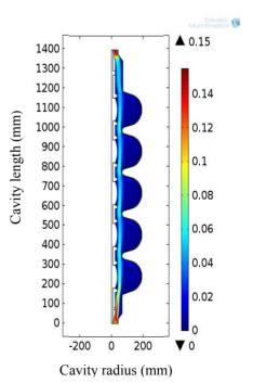
Figure 1: Electrolyte speed (m/s) distribution in an axisymmetric cut of a SPL five cell cavity assembled with its cathode.
