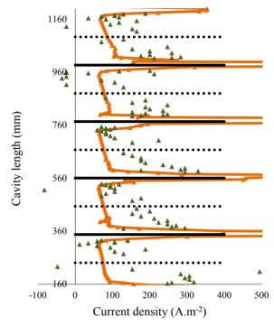
Figure 6: Current density distribution across the SPL five cell cavity for the second run. In green the experimental values and in orange the ones derived from the simulation data.
