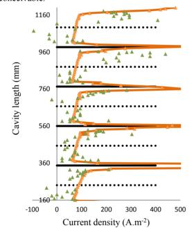
Figure 5: Current density distribution across the SPL five cell cavity for the first run. In green the experimental values and in orange the ones derived from the simulation data.
