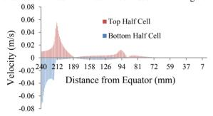
Figure 4: Electrolyte absolute velocity distribution at 5 mm from the cavity wall on a single cell. Negative velocity values are only for presentation purposes.
