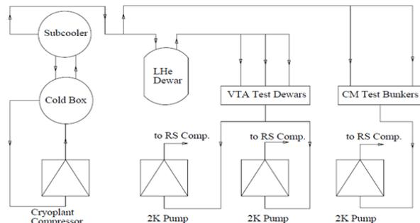
Figure 4: SRF Highbay cryoplant flow diagram.
