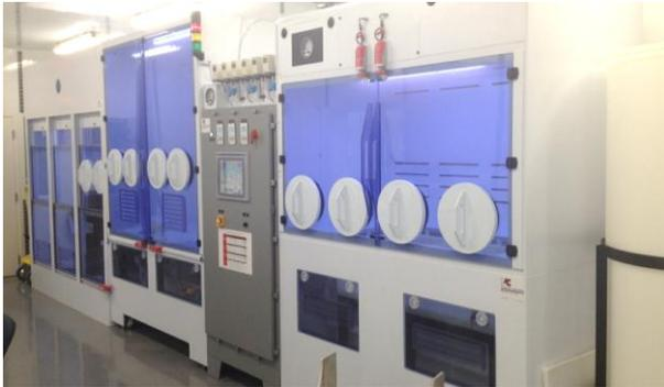
Figure 3: Automated chemical etch tools.
