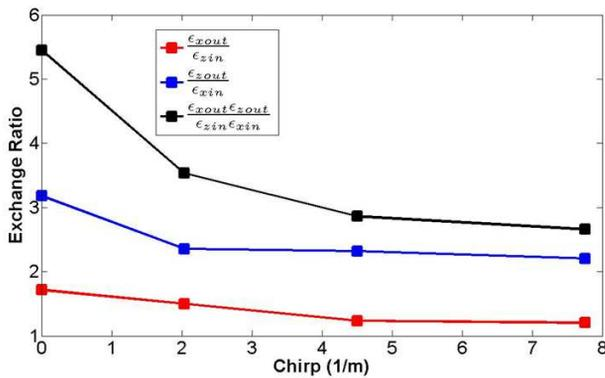
Figure 2: Measured value of the emittance exchange ratio and their products. As the RF-chirp increases, the ratio tends towards one. There is still some emittance dilution possibly due to second order effects and space charge
