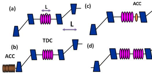
Figure 1: (a) Schematic of the classic double-dogleg emittance exchanger (b) Booster cavity before EEX to chirp and compensate thick-lens effect (c) Accelerating cavity inside the EEX to overcome thick-lens effect (d) Twin deflecting cavities to compensate thick-lens effect
