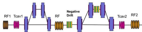
Figure 4: Emittance exchange scheme using two deflecting mode cavities and two chicanes
