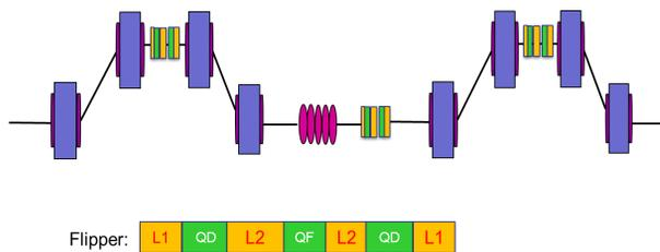
Figure 3: Emittance exchange scheme using one deflecting mode cavities and two chicanes. The strength of the cavity can be reduced by at least a factor of 2.
