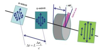
Figure 2: Illustration of pulse shaping through an  $\alpha$ -BBO crystal
