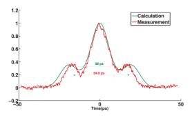
Figure 4: Longitudinal density perturbation generated and compared with the calculation.
