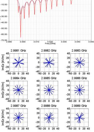
Figure 6: Input (red) and output (brown) couplers matching (top) and phase advance per cell (bottom) versus frequency.
