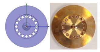
Figure 1: Regular cell design; 3D model (left) and copper piece (right) used in the creep test.
