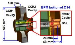
Figure 3: Button BPM mounted to a magnetic triplet in the 'inter tank section' between two CH modules.
