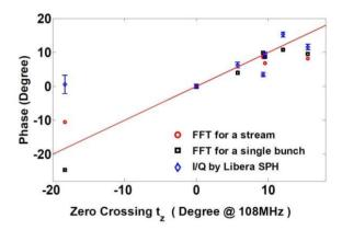
Figure 4: Time domain data compared to Libera SPH and FFT calculations for single bunch and streams of bunches.
