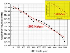
Figure 2: Variation of resonant frequency with changing the BCP depth of the SSR1 cavity.
