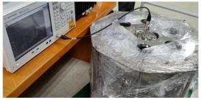
Figure 6: Clamp-up test for the SSR1 cavity prototype assembly.
