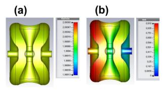
Figure 4: (a) temperature distribution in the SSR1 cavity by cool-down to 2 K and (b) the cavity deformation due to the temperature.
