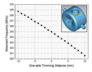
Figure 1: Variation of resonant frequency with changing the width of the outer conductor of the SSR1 cavity.
