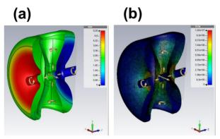
Figure 3: (a) SSR1 cavity deformed by vacuum pressure and (b) its electric field distribution.
