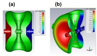
Figure 5: SSR1 cavity deformation at (a) 4 K and (b) 2 K.
