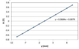
Figure 8: PMQ gradient (Hall probe measurement).
