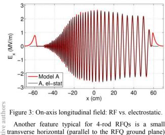
Figure 3: On-axis longitudinal field: RF vs. electrostatic.
