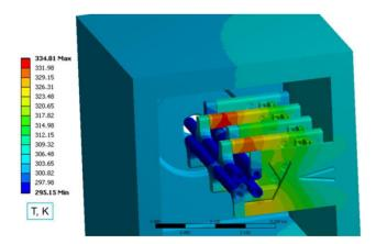
Figure 6: Temperature distribution from ANSYS [3].
