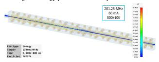
Figure 5: Particles in the LANL RFQ model with 60 mA.
