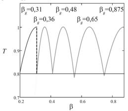
Figure 5: Slipping factor T versus beam velocity  $\beta$  in the high energy stage
