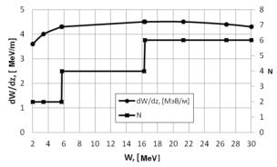
Figure 4: Dependencies of the minimum number of the crossed lenses and acceleration rate on the proton energy.
