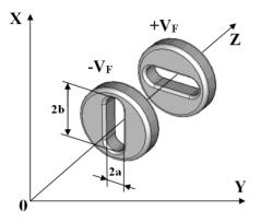
Figure 2: Two-electrode crossed lens
