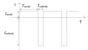
Figure 1: Typical periodic reverse current.
