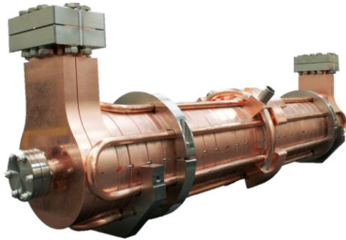
Figure 2: Picture of the PAL deflector after the final brazing and before installation.
