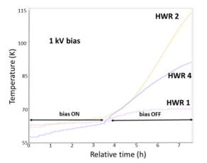
Figure 6: The effect of applying 1 kV bias on the  $2^{nd}$  and  $4^{th}$  cavities.
