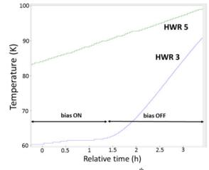
Figure 7: Non-sensitivity of the 5<sup>th</sup> cavity to DC bias application. The strong effect in the 3<sup>d</sup> cavity is shown for comparison.
