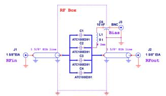
Figure 4: Electrical diagram of the final version of a 4 kW bias-T adaptor.
