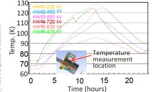
Figure 1: The couplers temperatures during operation of a 1 mA 3.6 MeV proton beam. The cavities voltages are indicated. The location where the temperature is measured is shown in the insert.
