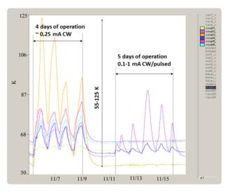
Figure 2: Daily variation of the warming rates during operation at the same field values. The couplers warmed up during day time operation and cooled overnight.
