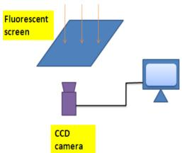
Figure 3: First step: use the fluorescent screen to get the distribution
