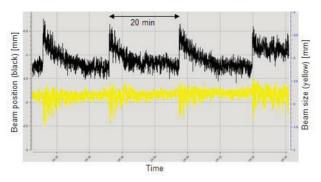
Figure 2: Beam position instabilities observed at the first YAG screen of Booster. The instabilities come from the linac beam but the source is still under investigation.
