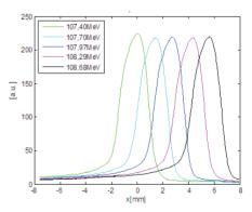
Figure 5: Beam position measurements taken at LTB-YAG02. Energy shifts produce a displacement of the beam in x-direction. The resolution is 0.45mm/MeV. At the Diagnostics Line the resolution is 20mm/MeV.
