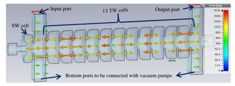
Figure 1: Structure of the hybrid buncher with the SW cell coupled in  $\pi$  mode and the following 13 TW cells in  $2\pi/3$  mode. The simulated electric field mode is shown as well. There is a 180° phase jump between the two sections.
