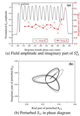
Figure 4: Measured results after tuning at 2997.1 MHz.
