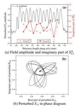
Figure 3: Measured results before tuning at 2997.1 MHz.
