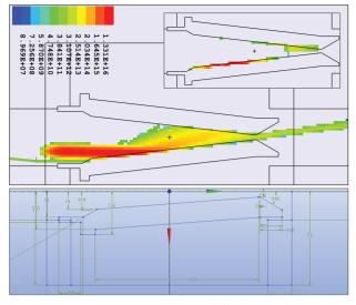
Figure 5: **Top Frame:** Side view of 62.5 mA 3.62 MeV proton flux density impacting on the beam dump. Onset figure indicates resulting heat map. **Bottom Frame:** Parametric representation of the beam dump.
