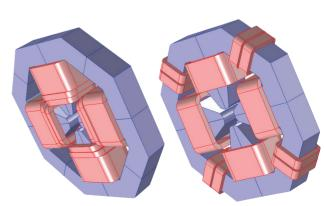
Figure 4: 3D models of proposed Steerer Coils In (Left) and Steerer Coils Out (**Right**). Coils are represented in red.
