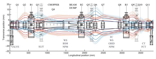
Figure 2: 2014 Layout proposed for the ESS MEBT; comprised of 11 quadrupoles 3 bunchers and 3 collimators [4]. Power density contours for x (*red*) and y (*blue*) are represented from dark ( $10^3$  W) to light ( $10^{-2}$  W) beam power contour lines extracted from TRACEWIN. Both axis are expressed in mm.
