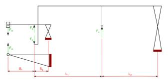
Figure 2: Scheme of force acting on the Tuner.  $L_1 = 350 \text{ mm}, L_2 = 350 \text{ mm}, S_1 = 67 \text{ mm}, S_2 = 30 \text{ mm}$
