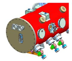
Figure 5: Access ports to the removable cartridge.
