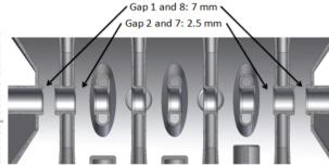
Figure 3: Optimized drift tubes for the sc CH-cavity.
