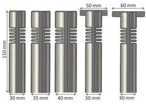
Figure 6: Layout of the different bellow tuners.
