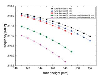
Figure 5: Frequency change through different bellow tuners.
