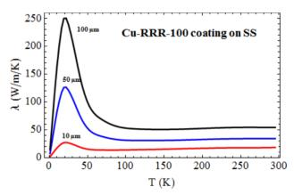
Figure 3: Thermal conductivity.
