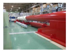
Figure 5: Picture of the ILC-type cryomodule assembly tool temporally stored in ATF hall.
