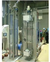
Figure 6: Cavity bed of vertical EP equipment.
