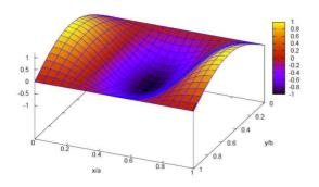
Figure 3:  $B_y$  normalized by the peak vale of the dipole mode  $TM_{210}$  cavity is shown in x-y plane. X and Y are also normalized with the cavity dimension in each direction and 0.5 corresponds to the center.
