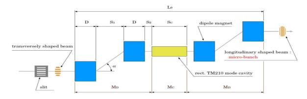
Figure 1: Schematic view of the EEX (Emittance EXchange) beam line which consists from two dogleg sections and one  $TM_{210}$  mode cavity. By passing a beam through the beam line, x and z phase-space distribution of the beam is exchanged by X-Z phase-space rotation.
