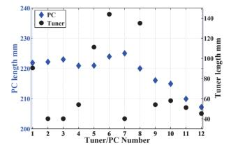
Figure 4: Final tuners and PCs length. The final PCs length are distributed  $\pm 10$  mm around the initial PCs length.
