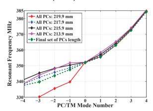
Figure 3: The measured dispersion diagram of PC  $_{-p}$  and TM  $_{01p}$  modes for different set of PCs length. The best confluence for constant PC length is at 217.9 mm.
