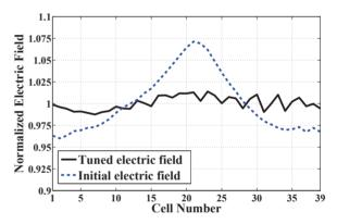
Figure 1: The initial (blue - without tuners and PCs) and the final (black) average electric field  $E_0$  of Linac4 DTL Tank1.
