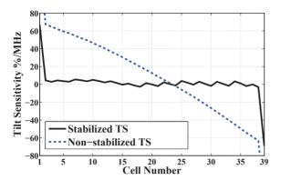
Figure 2: Comparison of stabilized (black) and non-stabilized (blue) TS of Linac4 DTL Tank1. The TS slope is reduced by factor of 28 using PCs.
