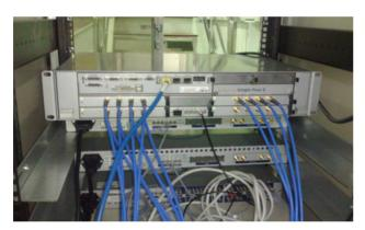
Figure 3: Libera Single Pass E connected to three stripline BPMs.
