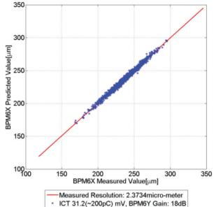
Figure 8: Achieved measuring resolution in horizontal plane using SVD calculation method.
