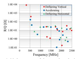
Figure 4: Mode spectrum of the normal conducting rfdipole cavity.
