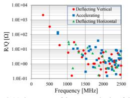
Figure 2: Mode spectrum of the superconducting rf-dipole cavity.
