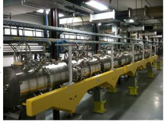
Figure 7: First 3 CCDTL modules in the Linac4 tunnel.
