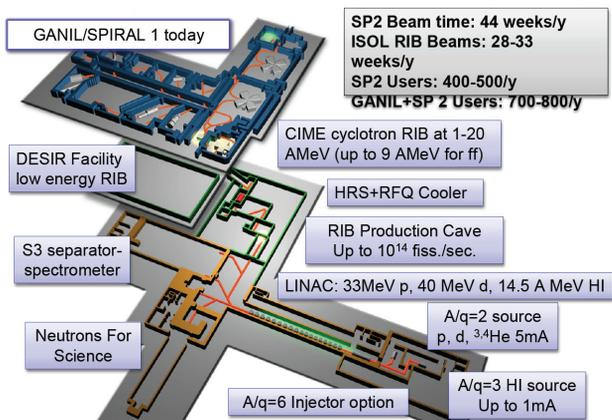
Figure 1: New and existing (in dark blue) facilities at GANIL site. Accelerator and stable beam physics in brown, RIB in green.
