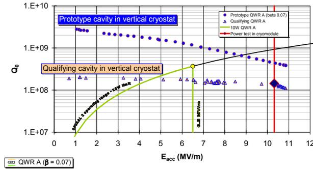
Figure 4: Prototype and qualifying QWR type A cavity in a vertical cryostat.
