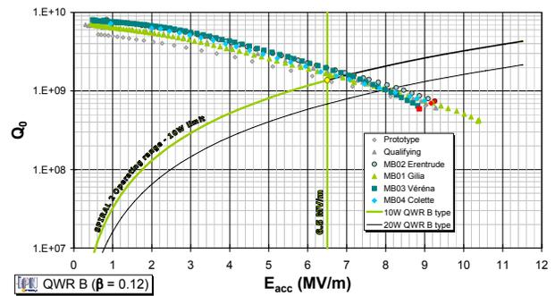
Figure 6:  $Q_0$  curve of the first type B cavities.
