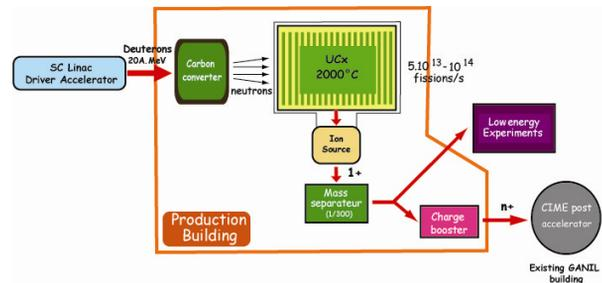
Figure 2: RIB production via the ISOL technique.
