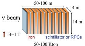
Figure 2: (Color) Schematic of the MIND concept for the Neutrino Factory.
