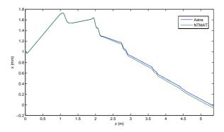
Figure 1: Tracking of an offset particle using Astra 3.0 and NTMAT. The initial kinetic energy is 10 eV, and the integration step size is 1 mm.
