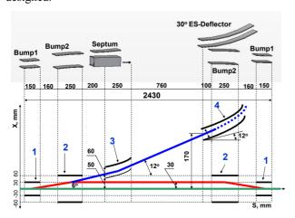
Figure 7: Position of the USR beam extraction elements.
