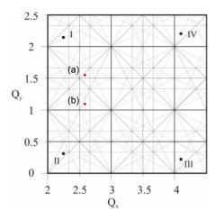
Figure 6: Tune diagram of the USR. (a) Betatron tune of the "round beam" operation mode ( $v_x$ =2.567 and  $v_y$ =1.576), (b) Betatron tune of the achromatic lattice used for short bunch operation mode ( $v_x$ =2.57 and  $v_y$ =1.16). The betatron tunes of the previous USR design based on 90° deflectors are indicated by I to IV.
