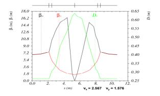
Figure 3: Beta-functions and dispersion in one USR cell for the round beam configuration.
