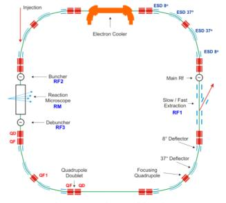
Figure 1: New layout of the USR.
