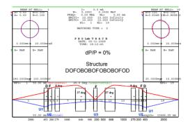
Figure 4: TRACE3D simulation of the 300 keV beam envelope in one quarter of the USR.
