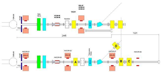
Figure 1: Schematic of the ALICE gun commissioning beamline (top) marking the position where diagnostic sections were removed and the booster linac added. The bottom shows the schematic of the extended ALICE injector up to the entrance of the first cell of the booster.
