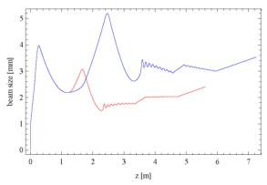
Figure 2: Transverse beam size (rms) along the existing (red) and extended (blue) injector beamlines.
