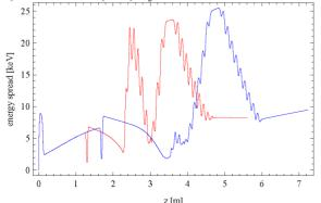
Figure 6: Energy spread (rms) along the existing (red) and extended (blue) injector beamlines.
