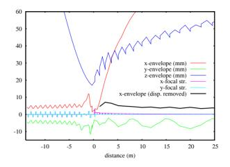
Figure 3: Beam envelopes through the injection line and into the cyclotron. Charge per bunch is 22 pC for a time average current 0.50 mA.
