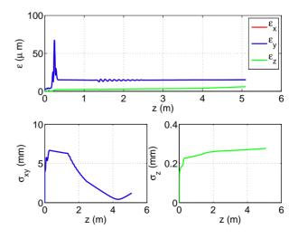
Figure 2: Top plot is the transverse emittance ( blue and red) and longitudinal emittance evolution along AWA beam line. Bottom plot is for the beam size and bunch length evolution.
