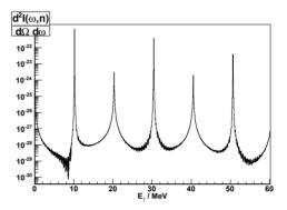
Figure 8: The photon energy distribution of radiation emitted by a 150 GeV electron passing through one section (1.79 m, 155 periods) of a helical undulator. The first harmonic occurs at a photon energy of 10.1 MeV.
