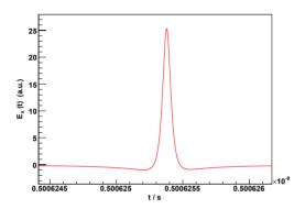
Figure 2: The calculated electric pulse due to an electron in a circular orbit. The observation point is in the same plane as the electron's path, so only the *x*-component of the electric field is present.
