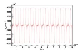
Figure 7: A portion of the *x*-component of the electric field, observed 10 m from the end of a 1.79 m helical undulator (155 periods).
