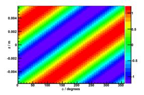
Figure 4: The radial component of the magnetic field in a helical undulator with periodicity 0.115 m, projected onto the surface of a cylinder of radius 0.0019 m.
