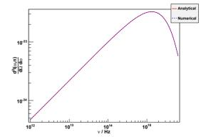
Figure 3: The differential power spectrum for an electron in a circular orbit, measured in  $J\,Sr^{-1}$ , radiated into unit frequency interval. The analytical and numerical curves agree within 0.05%.
