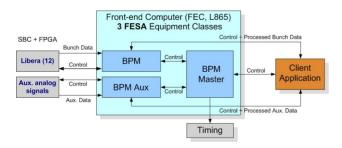
Figure 3: SIS-18 BPM system: FESA software layout.
