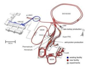
Figure 1: Layout of the FAIR facility including the existing accelerators UNILAC and SIS18.
