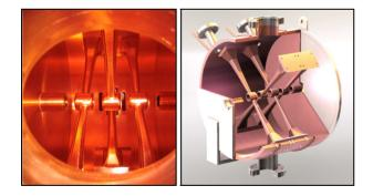
Figure 2: HINS RT-CH cavities: 3-spoke cavity photograph and 4-spoke cavity design rendering.
