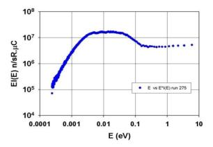
Figure 7: :EMS measured neutron flux from the cryogenic methane moderator.
