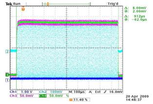
Figure 3: The 13 MeV Proton Beam Pulse as detected by 2 current transformers shown in red and green and an RF pickup shown in light blue.
