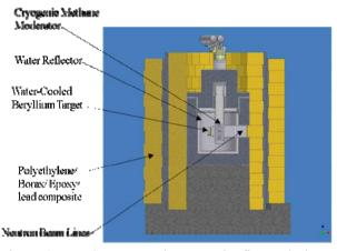
Figure 6: LENS target moderator and reflector design.
